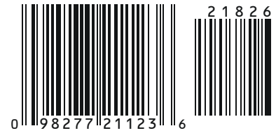
UPC A + Five-digit Supplemental (encoding 09827721123, supplemental = 21826)
