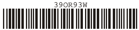
Code 39 (3-of-9 Code) (encoding 39OR93 with check character yielding a 2.32 inch wide symbol)
