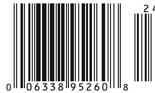
UPC A + Two-digit Supplemental (encoding 00633895260, supplemental = 24)
