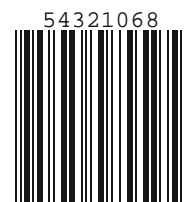
Interleaved 2-of-5 (encoding 54321068)
