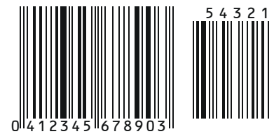
EAN + 5 Digit Supplemental (encoding 041234567890, supplemental = 54321)
